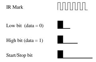
The high pulse illustrates six 38 kHz cycles.
